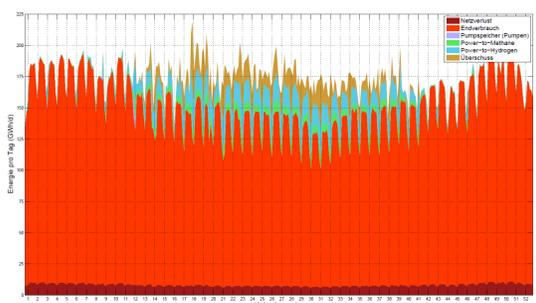
Figure 4: Modell of future energy supply and consumption in Switzerland. Excess energy is stored as gas. Model provided by SCS AG.
